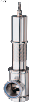
Safety valve DN 25 for liquids und gases (spring-loaded) with outlet thread DIN 11851
